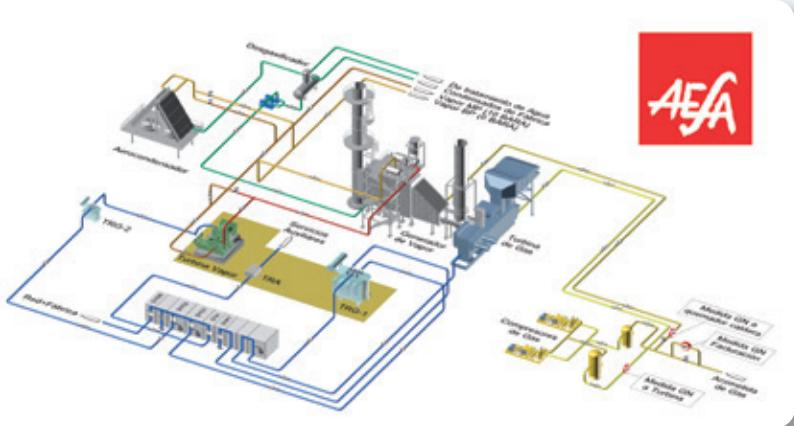
towards the boiler, and in the event of a high demand for steam the post-combustion burner starts operating. In the case of low steam demand, the by-pass evacuates the excess gases into the atmosphere.
